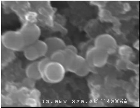
Figure 1. SEM image of spherical CEINPs
