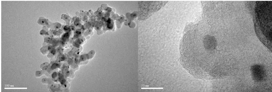
Figure 2. A: TEM overview of CEINPs, B: HTEM image of iron at carbon shell
