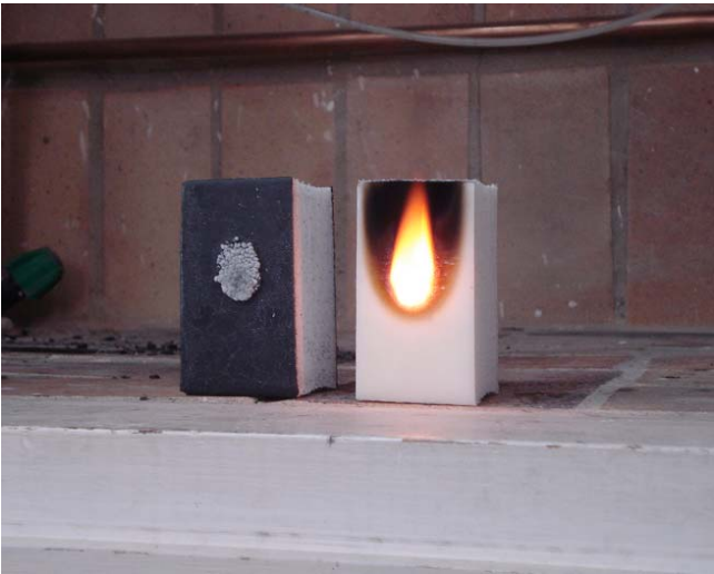
Figure 2. Flammability test for sandwich panels.
