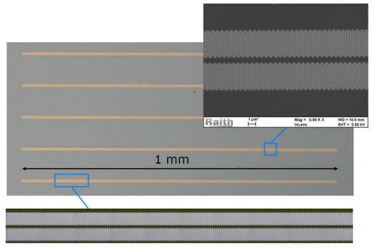
Figure 3. Hexagonal array of a 1mm-long, stiching error free photonic crystal waveguide written with MBMS stage technology.
