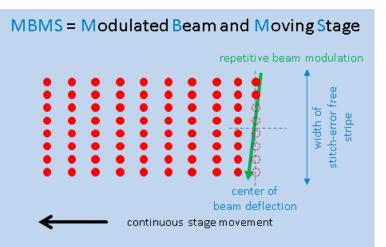
Figure 1. Exposure methodology of Modulated Beam and Moving Stage technology.
