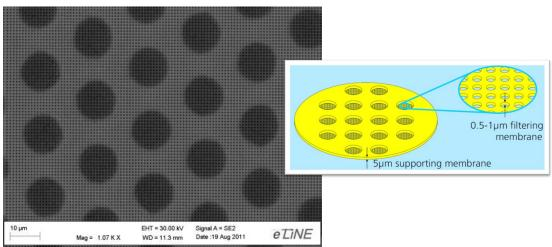
Figure 2. A micro filter featuring a 3mm x 3mm area circle array in a nickel membrane.
