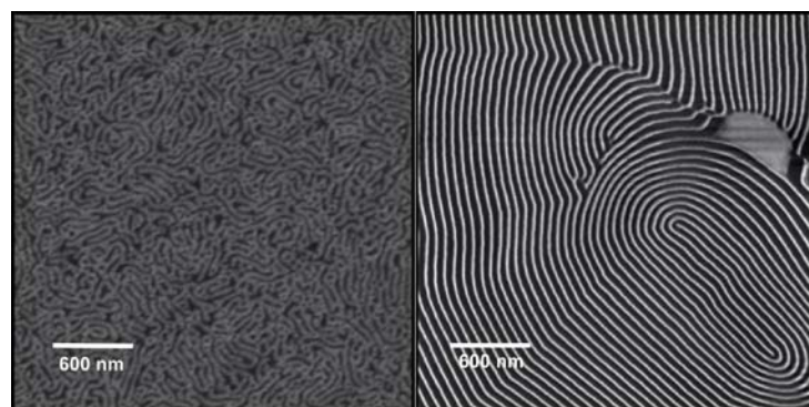
Figure 1. AFM phase images of copolymer A and B thin films after thermal annealing
