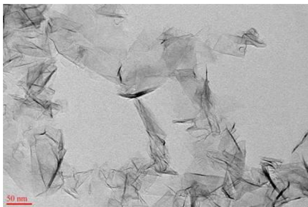
Figure 2: The TEM of graphene nanoplatelets from methane feed material
