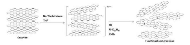
Schematic synthesis of graphene grafted via an in situ functionalisation of Na-reduced graphite.
