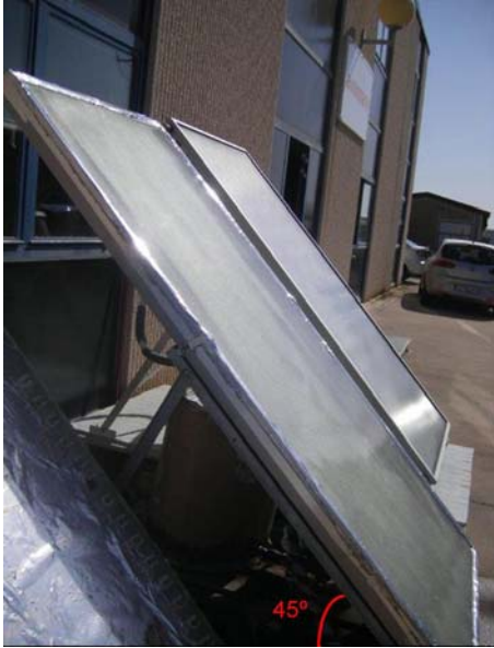
Figure2. Lateral view: ThermalCond collector (left); comercial collector (right).
