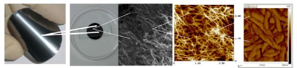
Figure 3: Processing of CNT into free-standing paper-like materials
