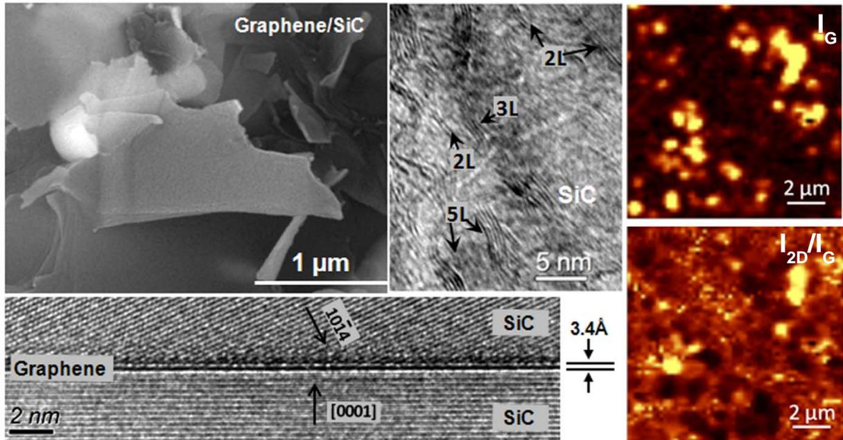
**Figure 1.** FESEM micrograph of the fracture surface of a graphene/ $\alpha$ -SiC composite where multi-layered graphene flakes are shown bending along grain boundaries, HRTEM examination showing few-layer graphene domains at different grain boundaries and Raman spectroscopy mappings on scanned areas of  $10 \mu\text{m} \times 10 \mu\text{m}$ .
