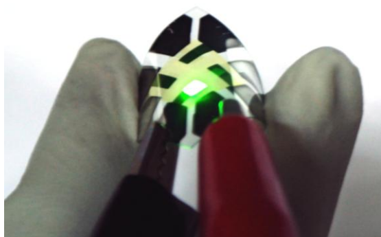
Figure 1. Flexible OLEDs using graphene anode. (a) Optical images of light emission from a flexible green OLED with a four-layered graphene anode doped with HNO 3 , (b) Performance of phosphorescent OLEDs with four-layered graphene and ITO anodes
