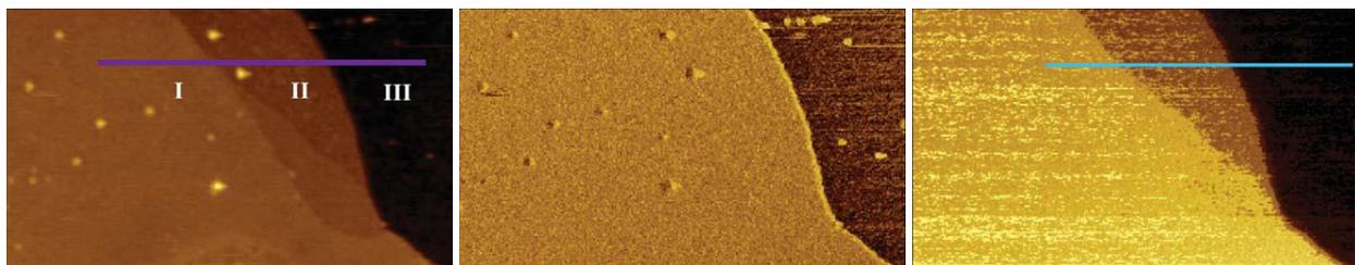
**Figure 2** Topography (left), Capacitance gradient ( $dC/dZ$ ; middle), and Surface Potential (Right) images recorded in single-pass Kelvin Force Microscopy (KFM) of few-layer graphene on silica surface.
