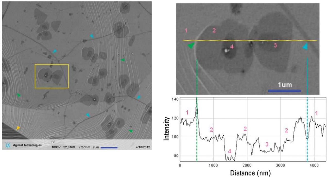
**Figure 1** left) A typical SEM micrograph of CVD synthesized graphene on Cu foil; right) magnified image of the yellow box in a) showing different contrast in certain areas; right bottom) the intensity profile along the yellow line in the top right image clearly displaying four plateaus representing monolayer, bilayer, trilayer and quadrilayer graphene.
