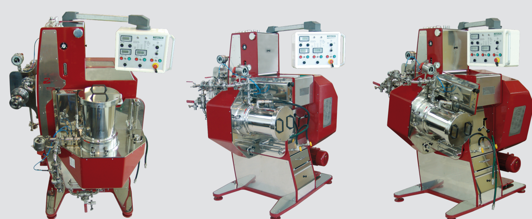
Figure 2 Agitator bead mill in positions for filling, operation and discharge
