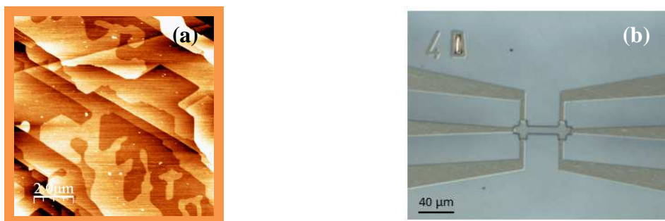
Figure 1: a) AFM image of SiC graphene grown on Si face (annealed under H 2 , growth at high T°C for 30 min under Ar); b) OM image of the graphene device geometry.
