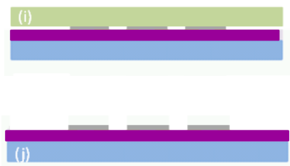
Figure 7: i) j) schematic drawing of structured graphene transferring on i) adhesion of graphene on tape onto 90 nm SiO 2 j) thermal release of tape
