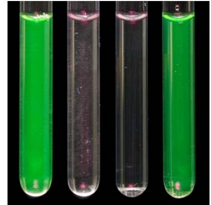
Figure 2. Left to right: C-LytA-GFP solution prior to binding to magnetic nanoparticles; two washes with 1M NaCl; elution of protein from the particles with choline.
