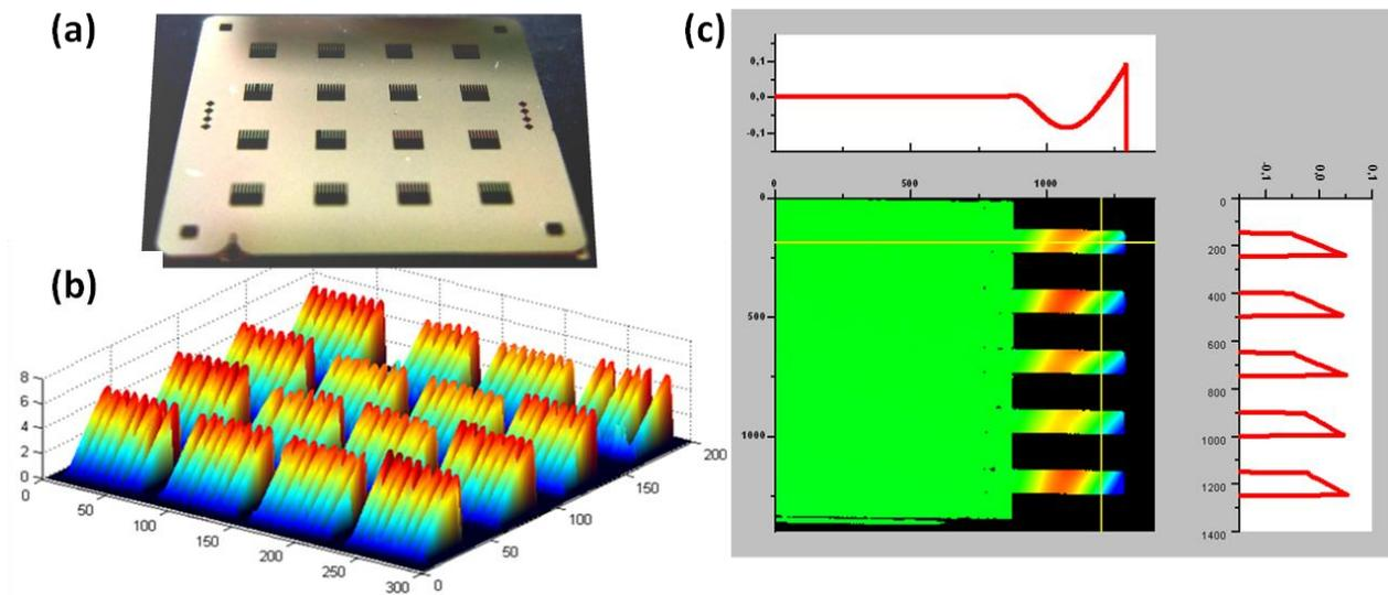
**Fig. 1** (a) Optical image of an 2D array of 128 microcantilevers arranged in 4x4 wells Each cantilever has 400 microns in length and 50 microns in width.(b) SCALA height image of the whole array.(c) SCALA vibration image of an array of 5 microcantilevers of the second vibration mode at 60 kHz.
