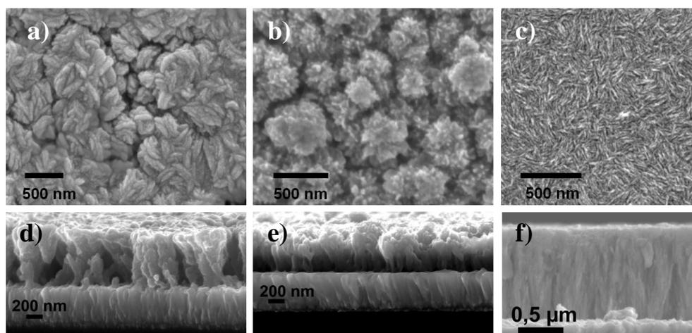
**Figure 1:** SEM micrographs of the top view (a, b and c) and cross sections (d, e and f) of ZnO films obtained under different electrodeposition conditions.
