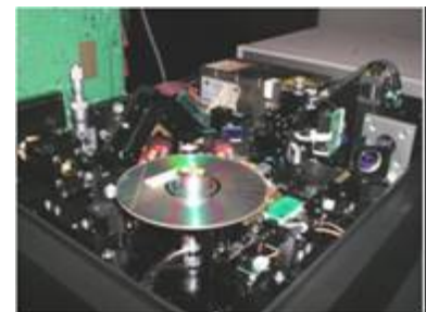
Fig.3 Collinear holography optical storage (Optware, Ecma standard).
