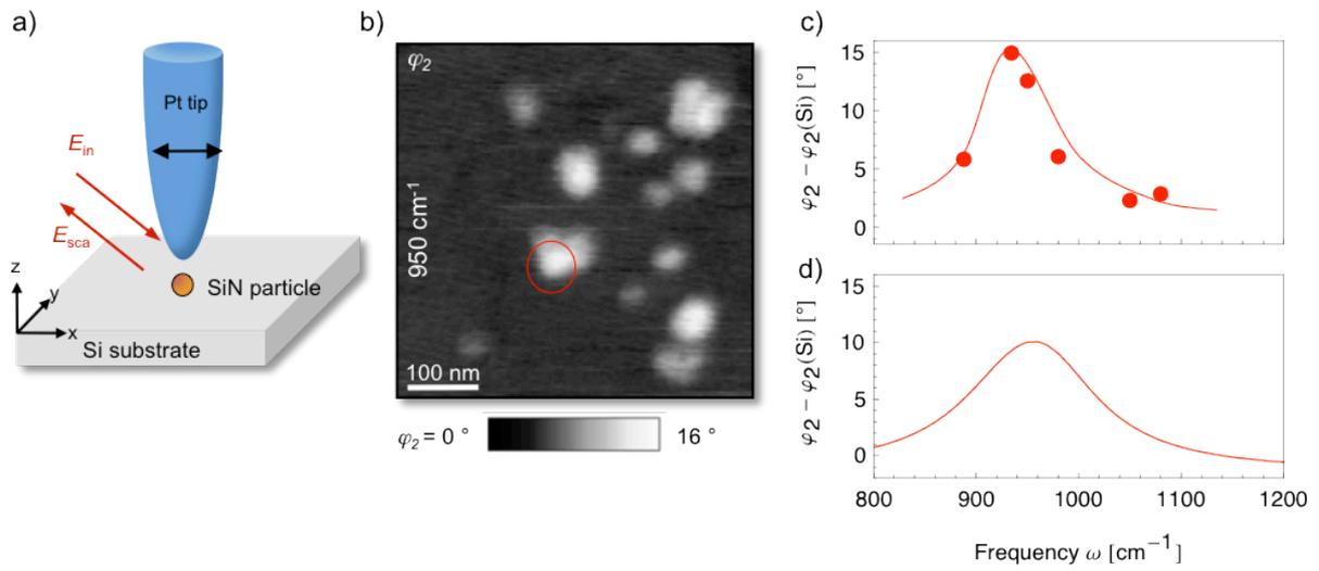
Spectral s-SNOM imaging of a 10 nm SiN nanoparticle. a) Experimental Setup. b) Experimental image showing an IR phase  $\varphi_2$  image recorded at  $950 \text{ cm}^{-1}$ . c) Measured and d) calculated near-field phase  $\varphi_2$  spectrum of the particle circled in b). The solid line in c) represents a guide to the eye.
