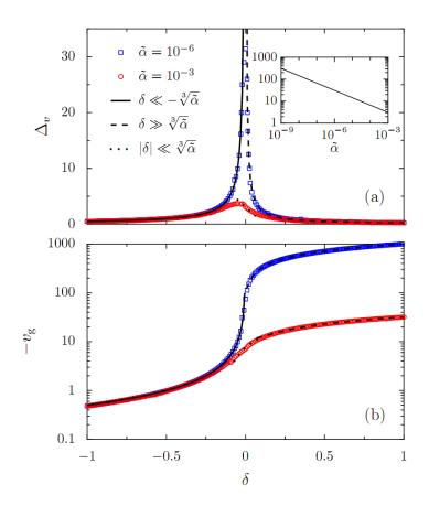
Fig. 2 Gap (a) and gate voltage position of the minimum gap in dimensionless units (b) as a function of the dimensionless distance from the transition point:  $\delta$ =F/F<sub>c</sub>-1, where F is the force acting on the rod, and F<sub>c</sub> is the critical force. One can clearly see a great enhancement of the gap of the order of 30 times the original value at the transition point. The red and blue curves correspond to different values of the non-linear coupling.
