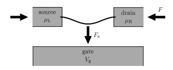
Fig. 1 Sketch of the considered system: a suspended doubly- clamped beam forming a quantum dot electrically connected to source and drain electrodes. The beam is capacitively coupled to a metallic gate kept at a voltage  $V_{g}$ , which induces a force  $F_{e}$  that attracts the beam towards the gate electrode. An additional, externally controlled compressional force F acts on the beam and induces a buckling instability
