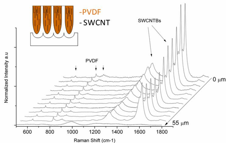
Figure 2. Depth profile Raman spectra of PVDF/SWCNT nanorods.
