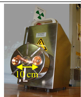
Figure 4: Picture of the dual X-ray source associated with the power supply.
