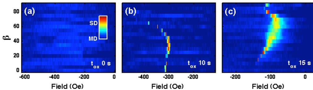
Figure 2: Single-domain/multi-domain existence map for samples with different degrees of crystallographic order as a function of applied field angle and strength: (a) fully epitaxial (1010) Co sample, and partially epitaxial samples, generated by  $SiO_2$  underlayer deposition of (b) 12s and (c) 15s duration.
