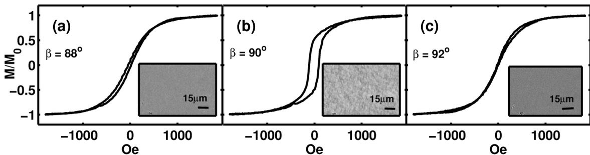
Figure 3: Hysteresis loop for a partially epitaxial sample, grown with  $t_{ox}=12s$ , for magnetic field orientations  $\pm 2^\circ$  away from the HA (a) and (c) respectively, and along the nominal HA (b). The inset figures show the remanent magnetization states taken by Kerr microscopy after applying a magnetic field along the corresponding field angle.
