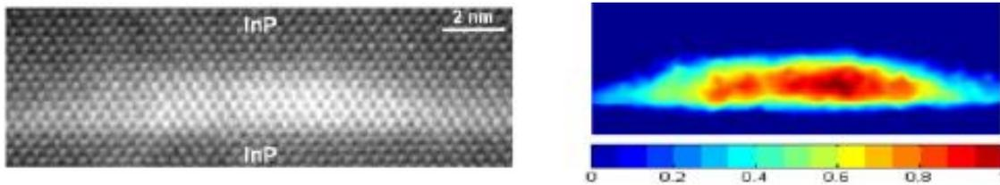
Figure 1. High resolution HAADF-STEM image of an InAs/InP quantum wire and its corresponding normalized integration intensity maps (reproduced from [4] with the permission of the copyright owner).
