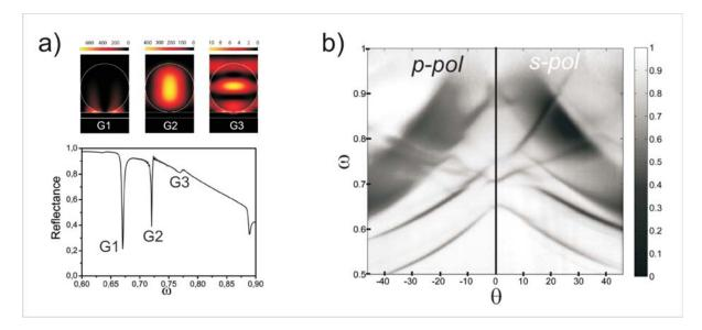
**Fig. 1** a) Normal incidence reflection spectrum for a dielectric array of 520nm diameter polystyrene spheres deposited on a gold substrate (bottom) and total field intensity profiles of the modes highlighted (top). b) Angle and polarization resolved reflection for the same sample.
