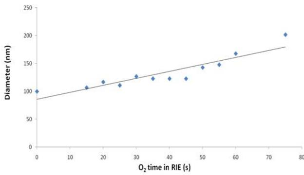
Fig. 4. Relation between holes diameter and O<sub>2</sub> plasma time in RIE
