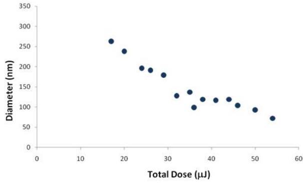
Fig. 2. Relation between holes diameter and exposure dose
