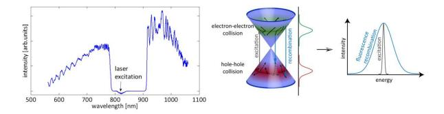
Left: Emission spectrum of a single graphene layer under picosecond excitation of 820 nm wavelength. Right: schematic representation of the 2D dispersion relation of graphene. The gray arrow shows the optical excitation of initially monoenergetic electron-hole pairs. Collisions lead to a broadening of the energy distribution as shown by the green and red curves. Recombination of shifted electron-hole pairs leads a broad fluorescence centered around the excitation energy.
