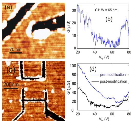
**Figure 3.** (a) AFM image of a  $\sim 65$  nm constriction formed in a bilayer flake using AFML and (b), its conductance,  $G$ , vs  $V_{bg}$  at 4.2 K. (c) QD formed in a bilayer flake using AFML, the entrances are initially  $\sim 150$  nm, these are then modified, as indicated by the blue arrows, using AFML to be  $\sim 50$  nm. (d)  $G$  vs  $V_{bg}$  at 4.2 K of the dot pre-modification (blue curve) and post-modification (black curve).
