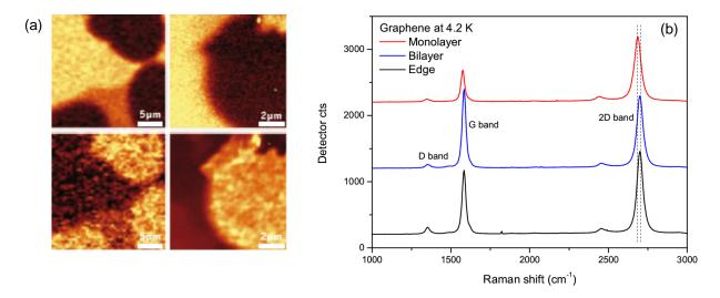
Figure caption: (a) Raman images of epitaxially grown Graphene layers, showing the SiC substrate (top) and the Graphene 2D band (bottom). Left images were recorded at 300 K, right images at 4.2 K. (b) Raman spectra recorded at 4.2 K, depicting (from top to bottom) monolayer and bilayer graphene, and the edge of the latter. The 2D band shifts by approximately 14 cm-1 at the transition from mono- to bilayer Graphene.
