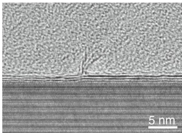
Fig. 2. Cross-section TEM image after MBE growth at 915 °C. The closed arrow points to the MBE-grown graphene layer and the open arrow points to the initial graphene formed by thermal decomposition of SiC.
