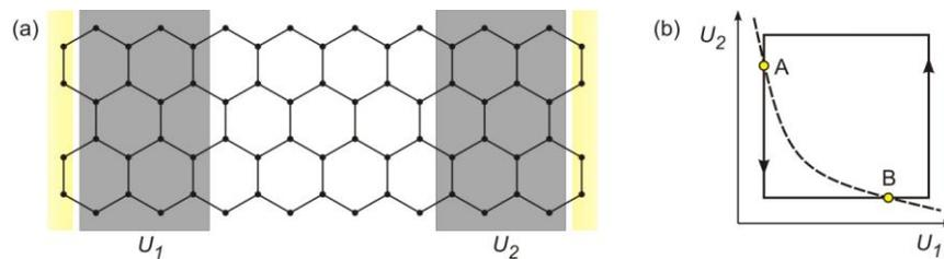
Fig. 1. (a) Schematic of the quantum pump ZGNR-based device (AGNR case is similar and not shown). Pumping is achieved by periodical variation of potentials  $U_1$  and  $U_2$ . (b) Typical pumping contour, schematic resonance line of conductance and two resonance points A and B.
