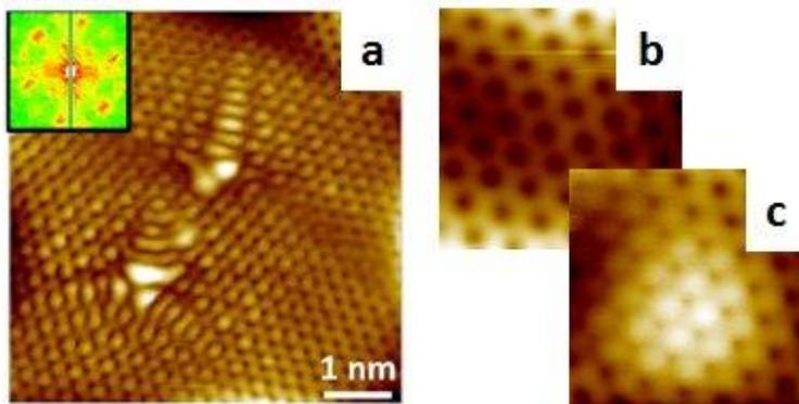
Fig. 1: STM constant current images of (a) scattering patterns at an adsorbate, (b) hexagonal contrast at 0.5 V, 0.1 nA (larger tip-sample distance), (c) trigonal contrast at 0.5 V, 5 nA (smaller distance).
