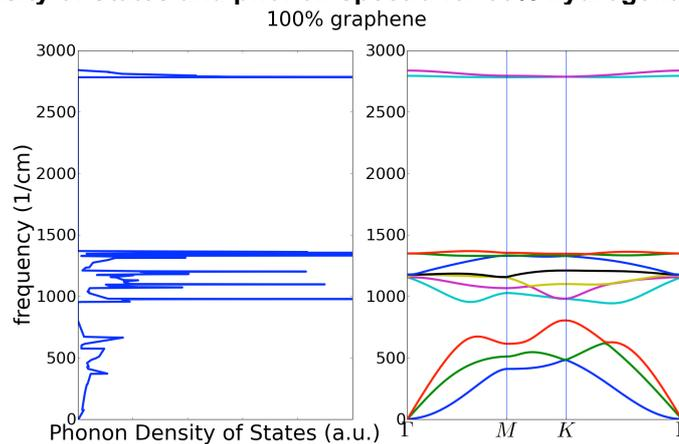
Fig.3: Phonon Density of States and phonon spectra for 100% hydrogenated graphene
