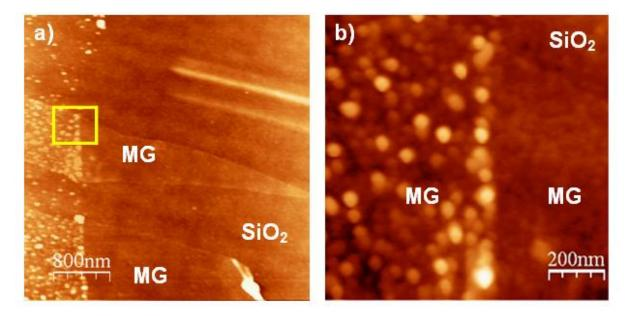
Fig. 1 AFM topography showing SiO<sub>2</sub> and MG regions after cleaning procedure. (b) The AFM topography showing the details of the interface between clean and dirty regions
