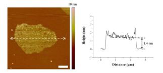
TappingMode AFM height image (3  $\mu$ m × 3  $\mu$ m, scale bar 500 nm) of a graphene sheet deposited from an ethanol solution onto a freshly cleaved mica surface. The height profile, following the white line on the image, shows the height of the graphene sheet to be ca. 1.4 nm which is equal to approximately 4 layers.
