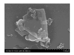
SEM image of graphene platelets stacked on top of one another, scale bar 1  $\mu$ m.
