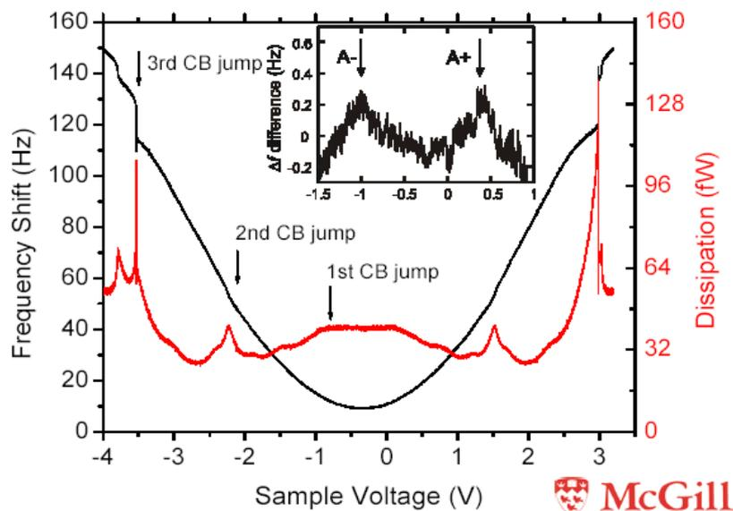
**Fig. 1:** Resonant frequency shift,  $f$ , and dissipated energy of the AFM cantilever as a function of the tip sample bias voltage. The arrows point to the sudden increases in the  $f$  caused by a single-electron charging in a QD and they appear as a peak in the dissipation at the corresponding bias voltage. The inset shows the magnified spectrum around the structures A+ and A-. Here, a fitted parabola to the spectrum around the minimum is subtracted. [1].
