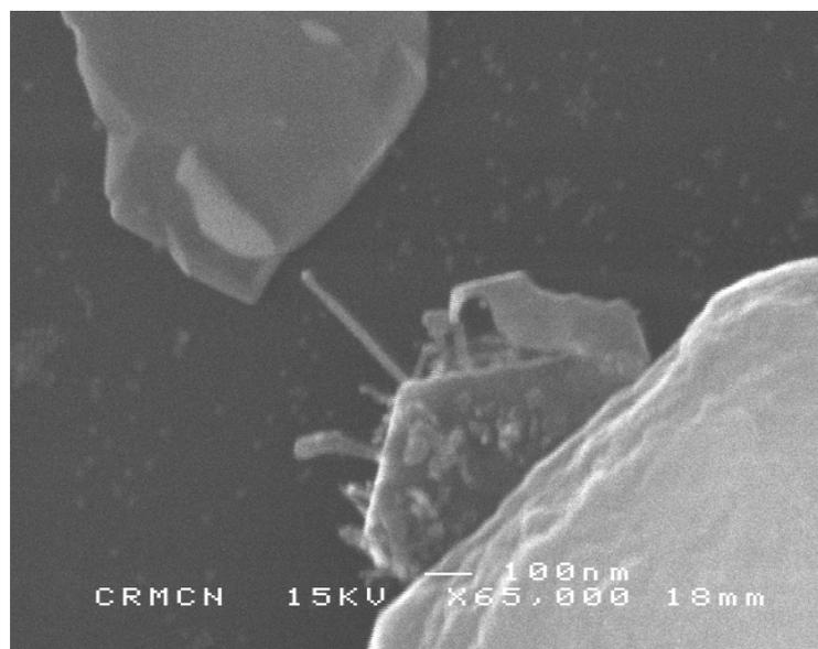
**Fig. 2 SEM image of horizontal growth of silicon nanowires.**
