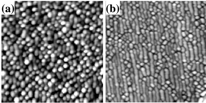
Fig. 1: Topographical AFM images of InAs grown nanostructures (a) dots. (b) wire-and-dot. Images sizes are  $1 \times 1 \mu\text{m}^2$ .
