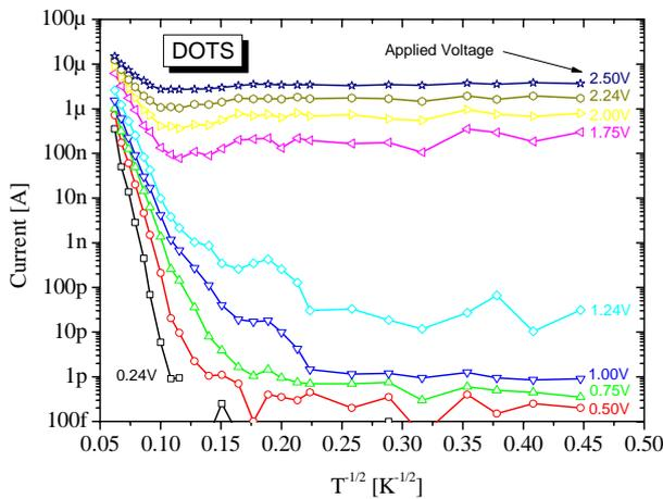
Fig. 4: Temperature dependence of the current for the processed devices (with dots) for a set of applied voltages.
