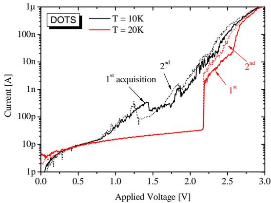
Fig. 2:  $I$ - $V$  curves at low temperatures for processed devices with dots. Fluctuations are observed in subsequent acquisitions.
