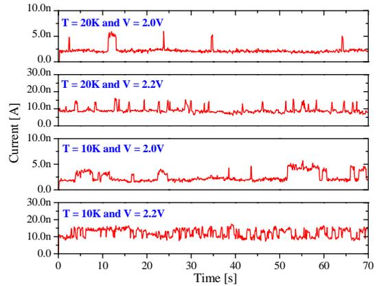
Fig. 3: Current vs time behavior for dots in a processed device. Switching between high and low levels indicates a signature of RTN.
