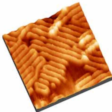
Low current STM image (41.5 x 41.5 nm 2 , 250 x 250 pixels) of a P3DDT film with submonolayer coverage on HOPG. V Bias = -1.45 V, I t = 5 pA, 300 K, base pressure < 6.10 -11 mbars.
