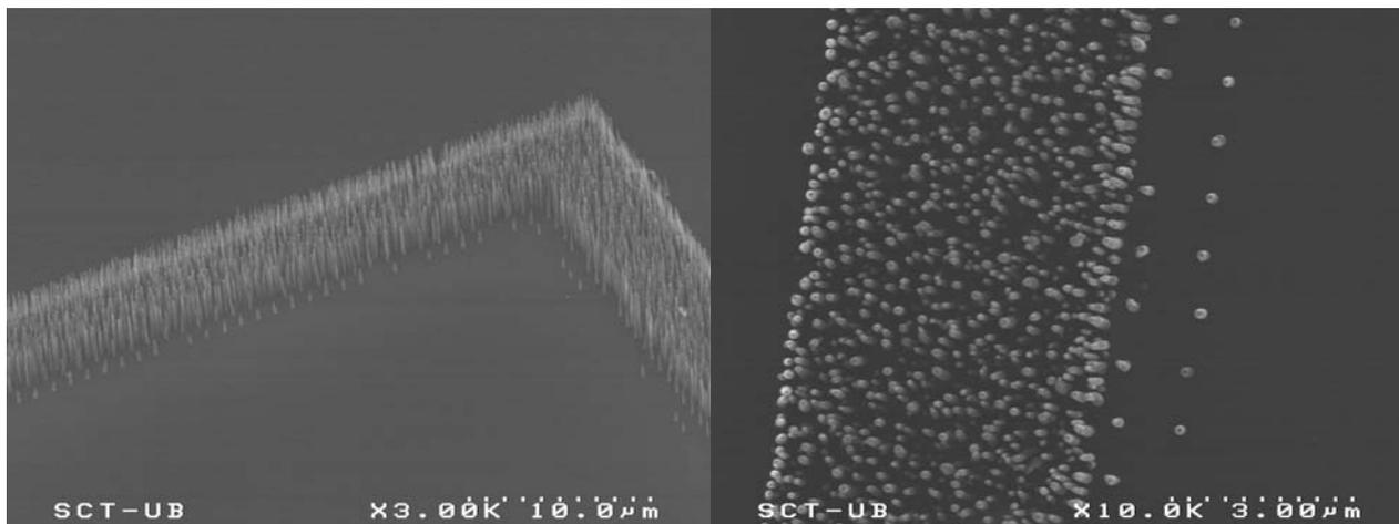
Figure 1: 45° tilted 30kV SEM (Hitachi S-4100) view of Ni dots matrix of CNTs surrounded by Ni nanoparticle frame.
