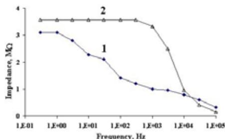
**Figure 3.** 1- impedance dependence on voltage frequency of Ge nanowire array, 2- equivalent RC scheme.
