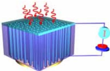
**Figure 1.** Scheme of photoconductivity measurement on Ge nanowire array.
