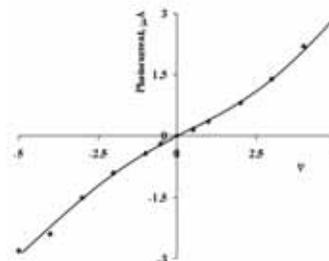
**Figure 2.** Photocurrent depending on voltage at laser intensity  $1400\text{mW/cm}^2$ .
