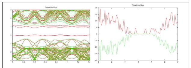
Fig.2. DFT Spin polarized up and down band structure calculations for diluted  $TiGa_{31}P_{32}$  showing an isolated intermediate band at the Fermi level (left) and the total density of states (DOS) of this structure (right).
