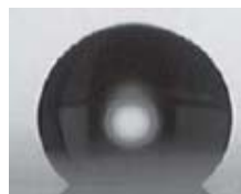
Figure 3. A water droplet on an ODS monolayer on porous alumina surface, showing the high contact angle of 146^\circ . Preparation conditions: 25 V, \text{H}_2\text{SO}_4 , pore widening 5 min.
