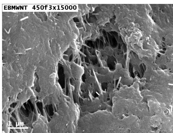
Figure 1: Scanning electron micrograph of CNT/PANI composite
