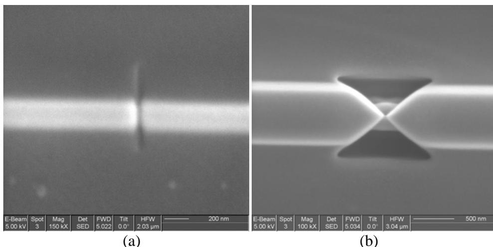
Figure: Platinum electrodes deposited and etched by FIB with nanogaps of (a) 40 nm and (b) 20 nm.
