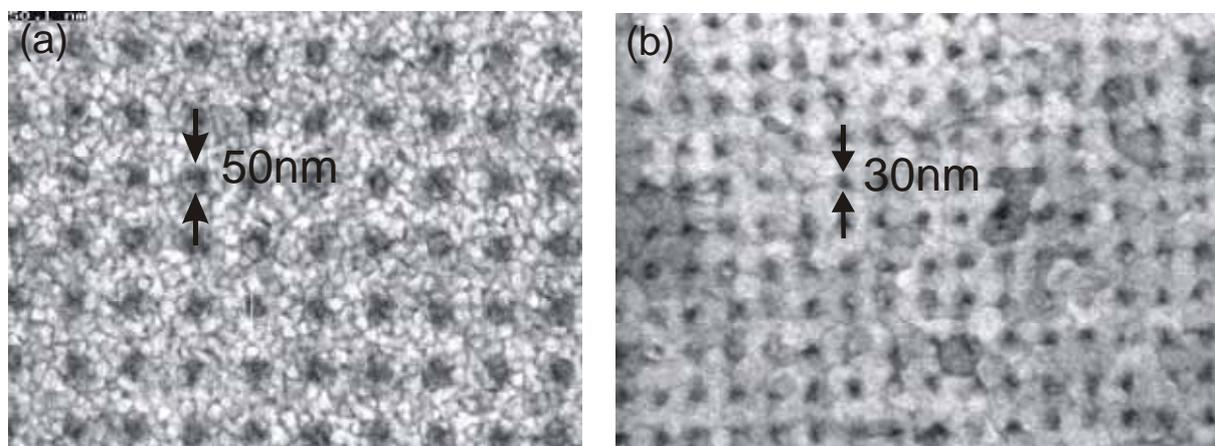
Figure 1: Scanning electron images of  $\text{TiO}_2$  dot structures appearing as round shadows on the bright platinum substrate. The dots in (a) are 50nm in diameter and have a distance of 75nm. The smallest  $\text{TiO}_2$  dot structures that were patterned reproducibly were 30nm in diameter with a distance of 45nm (b).
