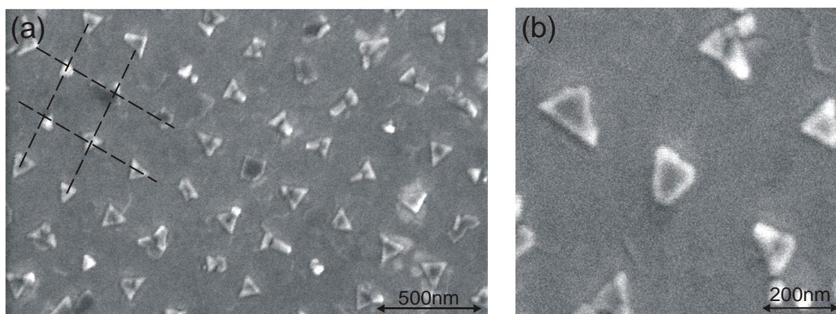
Figure 2: SEM images of separated PT nanograins deposited with a 1:30 diluted precursor solution on 100nm  $\text{TiO}_2$  seed structures. Here, the nucleation of the PT crystals exclusively took place on the  $\text{TiO}_2$  pattern whereas there was no crystallization at grain boundaries of the platinumized substrate. To point out the alignment of the PT crystals, grid lines are plotted in (a).
