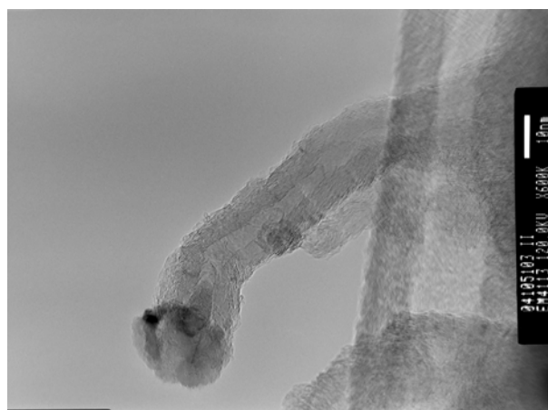
Figure 2: TEM micrograph of CNTs, obtained by plasma pulsed.
