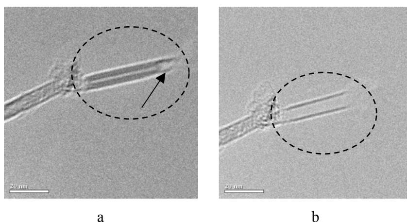
**Figure 2.** *In-situ* transmission electron microscopy of a degradation reaction of a multi-walled carbon nanotube under the influence of a strong electric field. (a) The open end of a multi-walled nanotube (see arrow), that had been broken-off before, imaged while emitting 8  $\mu\text{A}$  of current at 350 V extraction voltage. (b) The inner walls of the nanotube were removed/destroyed (encircled) and the nanotube continued emitting current of 3  $\mu\text{A}$  at 360 V.
