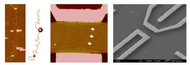
Gold nanoparticles funtionalized with defined short DNA sequences coupled to the complementary region along a long DNA molecule (left). An individual DNA molecule positioned by self-organization using a flow chamber into a prestructured electrode gap of 3 micron (center). SEM of an individual DNA structure imobilized in an extended state on a microelectrode arrangement by a modified droplet method prior to metal nanoparticle labeling (right).
