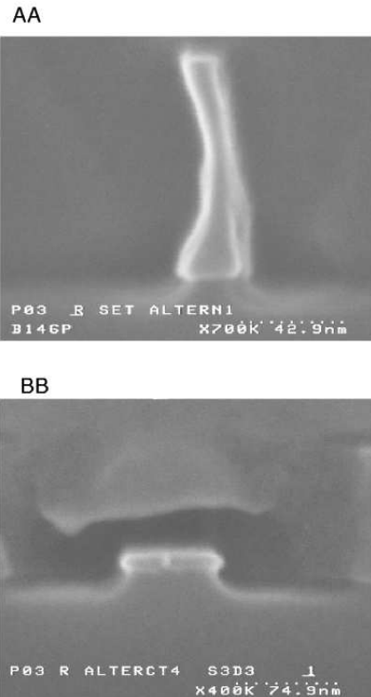
Figure 2: Top: SEM image of the gate along the AA axis (see Fig.1), after resist trimming and etching. The gate length is 20 nm at its base. Bottom: SEM cross section of the wire along the BB axis.
